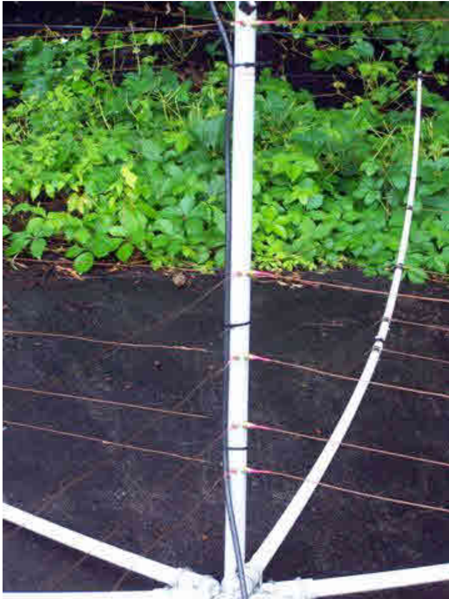
Close up of element wires as they attach to the spreaders. Note that driven and reflector elements are color coded at the ends of the element wires
